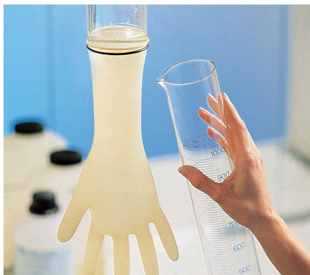
Water retention test
